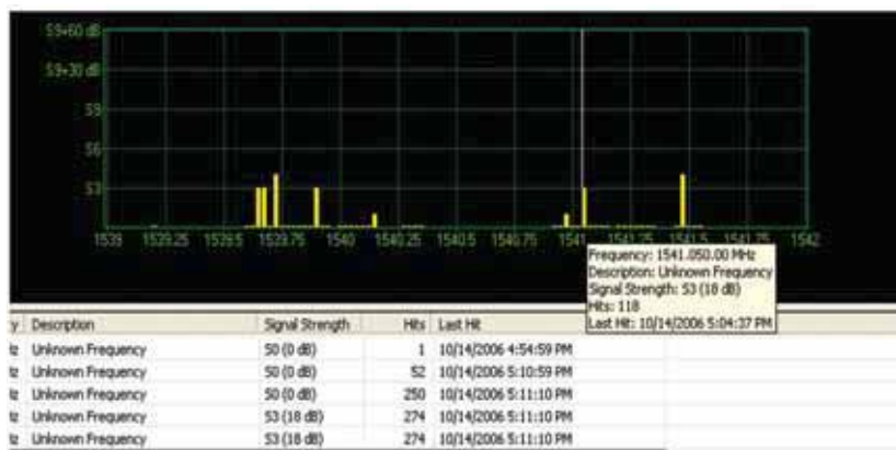
● Fig. 4: The cursor display dialogue when you hover over the spectrum chart plot.
